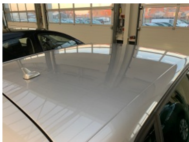
Roof - Hail damage
